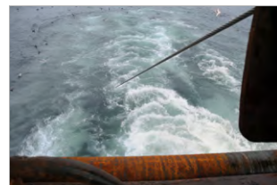
Figure 8. Trawl cables with steep descent directly behind vessel. Warps were in prop wash, which kept the birds away from the warp cables.
