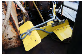
Figure 1. The Acoustic receiver that obtains a signal from the transducer mounted on the trawl headrope. This “fish” is deployed alongside the vessel off of a boom, and set about 10-15 fa deep.
