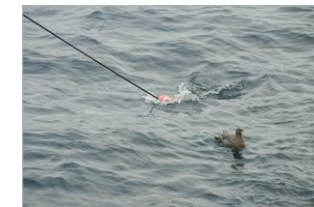
Figure 11. Float mounted around the paravane cable, able to move freely along the cable itself.
