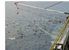
Figure 12. Streamer lines strung along the paravane cable boom.
