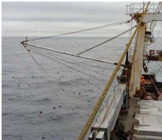
Photo 1: Field biologist Jeff Pesta conducting a seabird/paravane interaction session. The paravane cable runs down into the water from near the end of the boom (and back to the vessel under the boom). All other lines control the boom or are used to deploy and retrieve the block used to deploy the paravane. Very few interactions were recorded with these lines. Note the gull perched on the boom. © Todd Loomis, Cascade Fishing.
